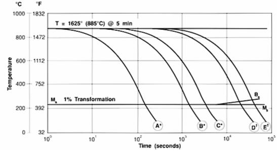
Partial continuous cooling curve-AerMet 100 alloy
