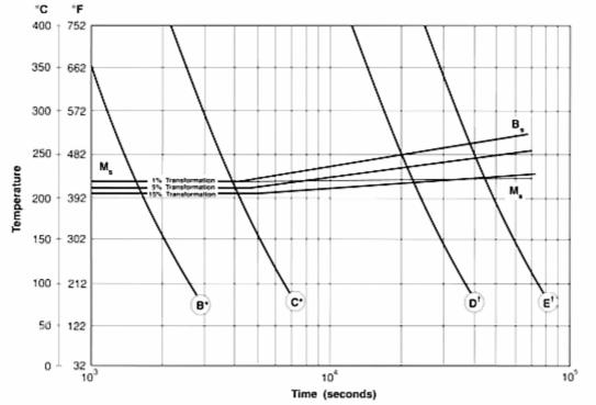
.12" (3 mm) diameter x .39" (10 mm) rod heated to 1625"F (885"C) at 360"F (200"C) per minute held at 1625"F (885"C) for 5 min quenched with helium gas.
